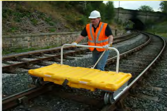
LT1000P – Combined polymer HDPE and aluminium deck construction is easy to handle very durable and high visibility.
