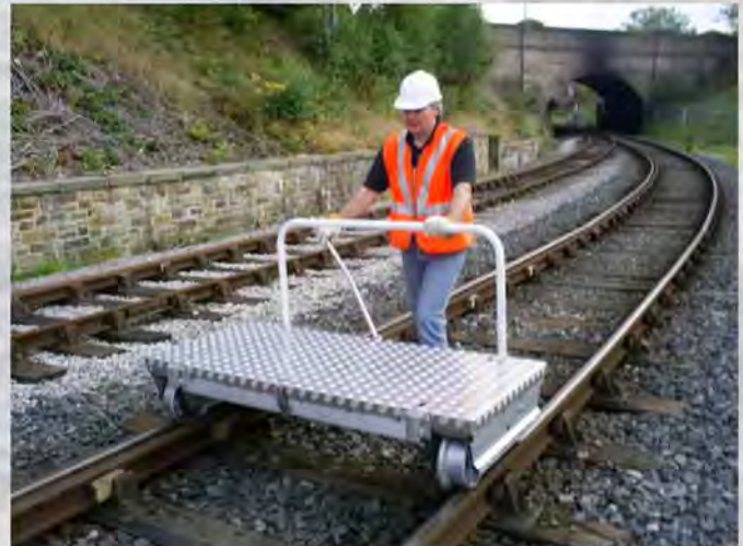
LT1250A – All aluminium deck construction is lightweight, strong and heat resistant.
